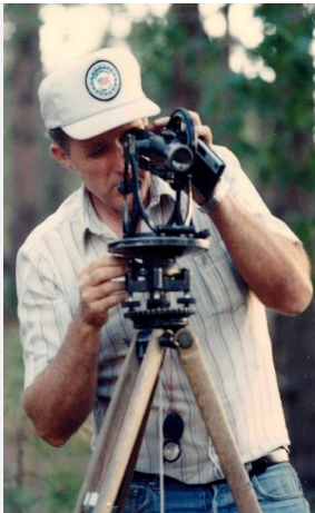
This is Kent with his transit, taking measurements and laying out the camp property and infrastructure probably around 1981.
